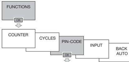
The menu PIN CODE allows you to lock the clock keyboard.
