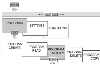
The number of free program steps is displayed. Press **ok** to validate. The buttons **+** and **-** allow you to scroll the programme steps. The button **ok** allows you to select the programme step to be modified.
