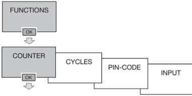
The first line indicates the number of operating hours of the output. The second line indicates the number of time changes (ON then OFF) done by the output. The buttons + or - allow you to scroll the various indicators.
